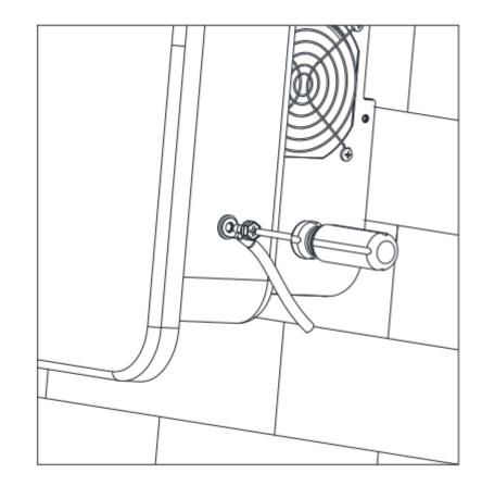
Recommended minimum cross-section of the grounding wire 6 mm2\*
