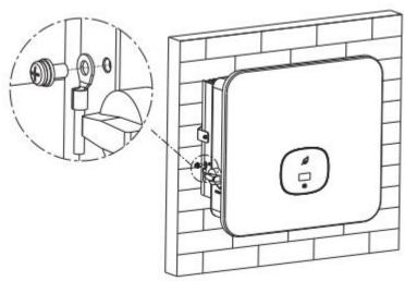
Recommended minimum cross-section of the grounding cable 6 mm2\*
