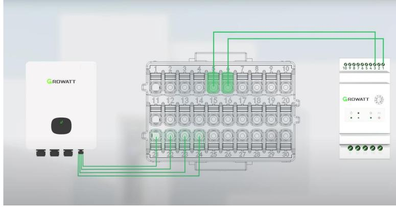
Standard length of the included Smart Meter communication cable is 15 m, can be extended up to 100 m
